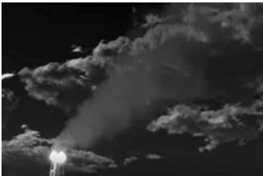
Figure 1. Image capture from a video of a conventional air flare taken by an OGI camera.
