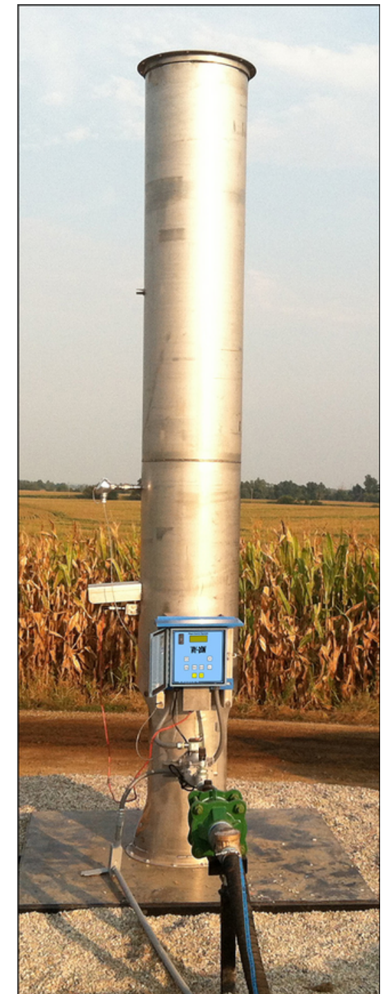
A Cimarron enclosed combustor device (ECD), one of the Company's 10 EPA certified models, installed in Illinois and equipped with a proprietary burner control device.
