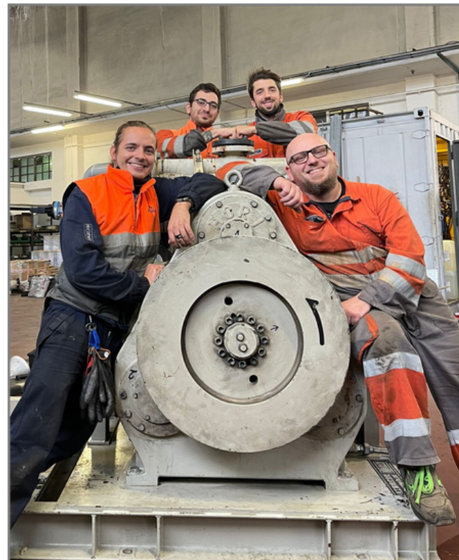
A team of Cimarron technicians at our facility near Pisa, Italy. They are refurbishing a Hori vacuum pump for a Carbon VRU application.
