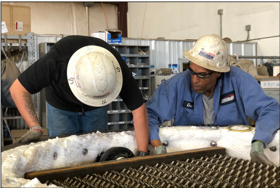
Technicians in Norman, OK are installing a high destruction efficiency burner in an EPA-approved enclosed combustor (one of 10 models).
