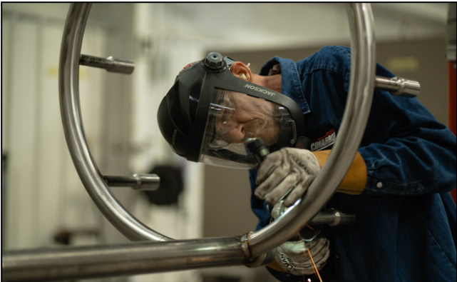
A welder at our plant in Norman, in Oklahoma, assembling a stainless steel smokeless flare tip.
