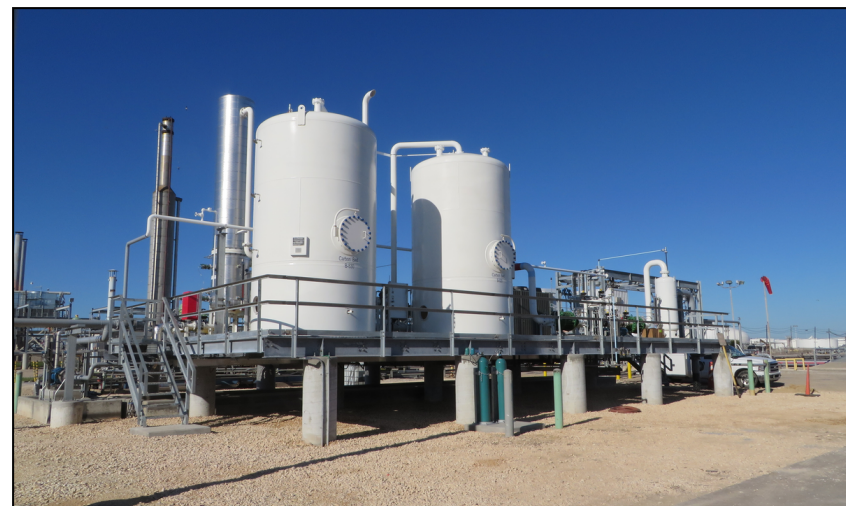
Our Carbon-based Vapor Recovery Systems capture 99.9%+ of vapors in liquid-loading terminal applications
