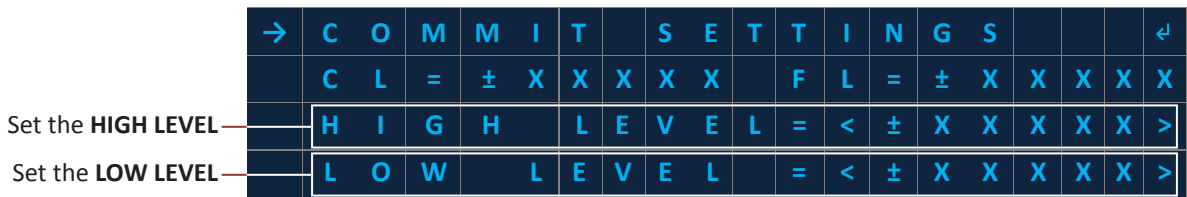
Image 2.8.3 • Set the process HIGH and LOW levels
